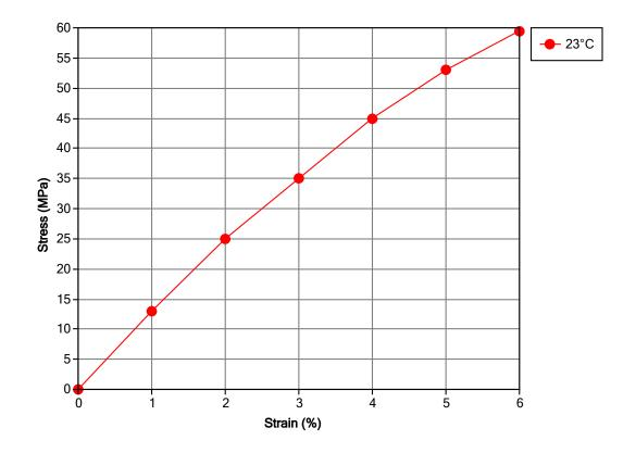
Secant Modulus vs. Strain (ISO 11403)
